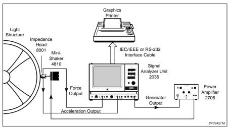
Fig. 3 Set-up for mechanical impedance and mobility measurements
