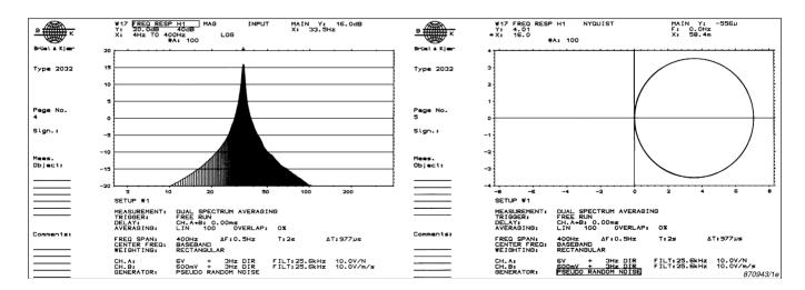
Fig. 4 The mechanical mobility function of a soft rubber material. The function is displayed as magnitude v. frequency (left) and real part v. imaginary part (a Nyquist plot, right)
