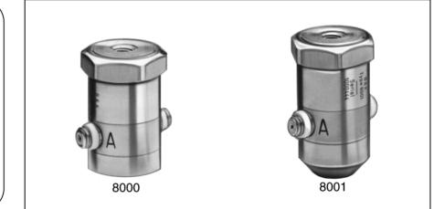
Impedance Heads Types 8000 and 8001 offer a way to measure the applied force and response at a point on a light structure. Simultaneous measurement of both of these quantities can provide data on the mechanical mobility and impedance of the structure at the point of interest. These measurements form the starting point of investigations into other dynamic properties such as accelerance, compliance, damping, loss factors and resonance frequencies.
