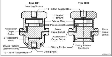
Fig. 2 Schematic drawings of Types 8000 and 8001
